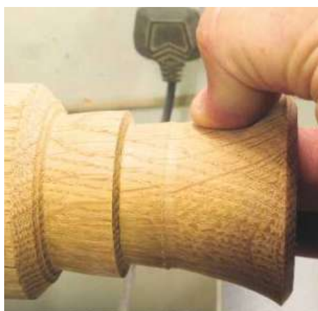
▲ Pic.14 There is no better gauge for measuring the wall thickness than your fingers. You can go back into the centre if you haven't got the shape quite right, as long as the base isn't too narrow
